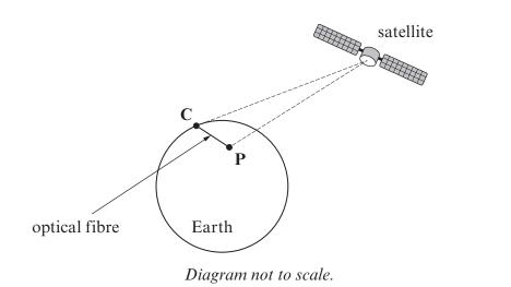
(a) The frequency of infra-red waves used in the optical fibre is 4 × 10<sup>14</sup> Hz and their wavelength is 5 × 10<sup>-7</sup> m.
