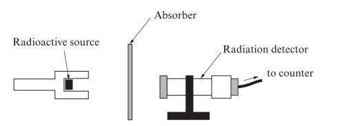
A number of different absorbers are placed, one at a time, between the detector and the radioactive source.
